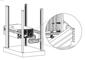
Install two M6 cage nuts into the vertical rail to which the cable arm is to be attached.
